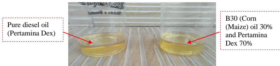
Fig. 2. Fuel samples. a) Pure diesel oil, b) Corn (Maize) oil B30
