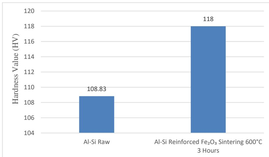
Fig 2. Comparison of the hardness of Al-Si alloy
