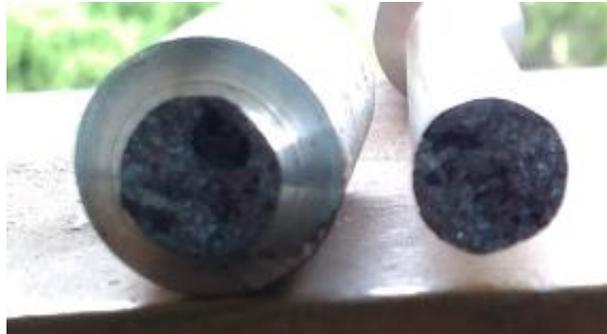
Fig 6. Morphology of Al-Si alloy reinforced by  $\text{Fe}_2\text{O}_3$
