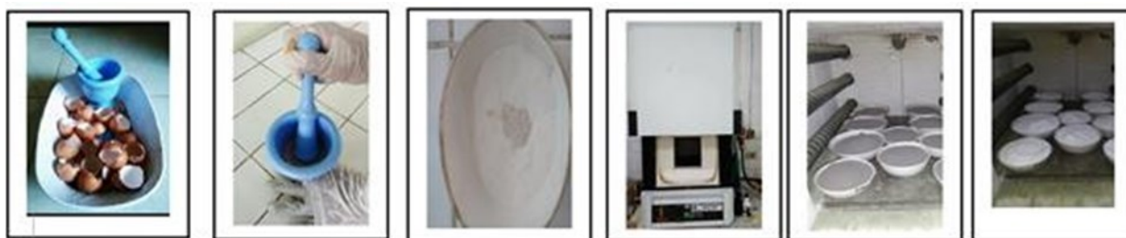
Figure 1. The synthesis scheme of CaO heterogeneous catalysts from pure breed chicken eggshells.
