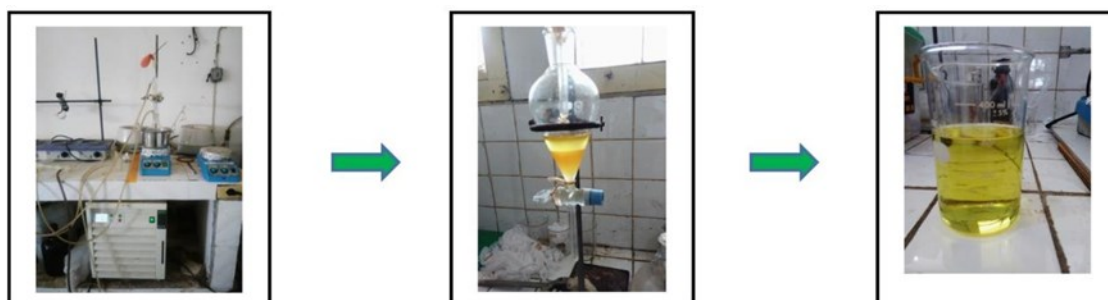
Figure 2. Preparation scheme of biodiesel made from waste cooking oil using CaO heterogeneous catalyst.
