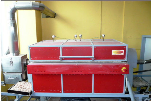
Fig. 2. Laboratory rotary kiln for lightweight aggregate production
