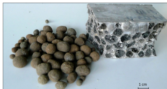
Fig. 4. Low strength lightweight concrete specimen and aggregates LA
