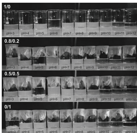
Fig. 4. Dispersions of composite zein/shellac (Z/S) nanoparticles of different Z/S mass ratio (1/0, 0.8/0.2, 0.5/0.5 and 0/1), and of different pH (3–11).
