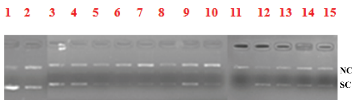
Fig. 1. a) Gel electrophoresis of copper(II) complexes (40 \mu M) in buffer containing 50 mM Tris/HCl/50 mM NaCl (pH 7.2) in the presence of ascorbic acid at 37 °C. Lane 1: DNA control; lane 2: DNA + ascorbic acid; lane 3: DNA + ligand HL+ ascorbic acid; lane 4: DNA + ligand H(L1)+ ascorbic acid; lane 5: DNA + [Cu(L1) 2 ] + ascorbic acid; lane 6: DNA + [Cu(L1)(phen)]Cl + ascorbic acid; lane 7: DNA+[Cu(L1)(bpy)]Cl + ascorbic acid; lane 8: DNA + ligand H(L3) + ascorbic acid; lane 9: DNA + [Cu(L3) 2 ]Cl + ascorbic acid; lane 10: DNA + [Cu(L3)(phen)]Cl + ascorbic acid; lane 11: DNA + [Cu(L3)(bpy)]Cl + ascorbic acid; lane 12: DNA + ligand H(L2) + ascorbic acid; lane 13: DNA + [Cu(L2) 2 ] + ascorbic acid; lane 14: DNA + [Cu(L2)(phen)]Cl + ascorbic acid; lane 15: DNA + [Cu(L3)(bpy)]Cl + ascorbic acid.
