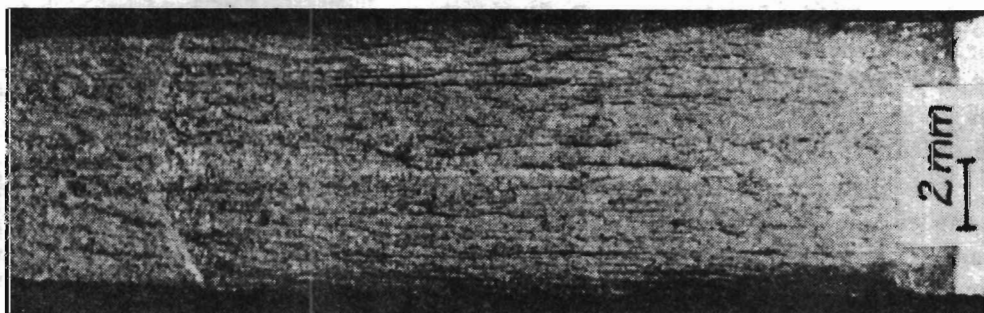
Fig. 3. Microfractograph of a SEC specimen tested without overloading
