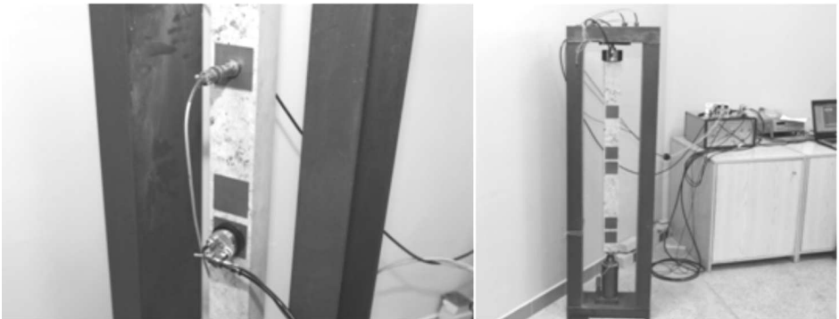
Fig. 4. The test stand for endurance tests using the SAS System
