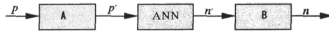
Fig. 3. A mathematical scheme of a neural model of a flying object; \mathbf{p} – vector of input signal [V_i, \delta_{hi}, \Delta\delta_{hi}, \dots] , \mathbf{p}' – vector of normalised input signal, \mathbf{n}' – vector of normalised output signal, \mathbf{n} – G -loads vector [n_{xi}, n_{yi}, n_{zi}] , \mathbf{A} , \mathbf{B} – matrices of signal transformation
