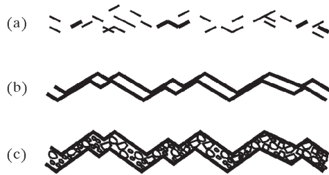
Fig. 25. The basic mechanisms occurring at brittle interfaces: (a) decohesion; (b) interaction of interlocked asperities; (c) formation and shearing of the third body layer
