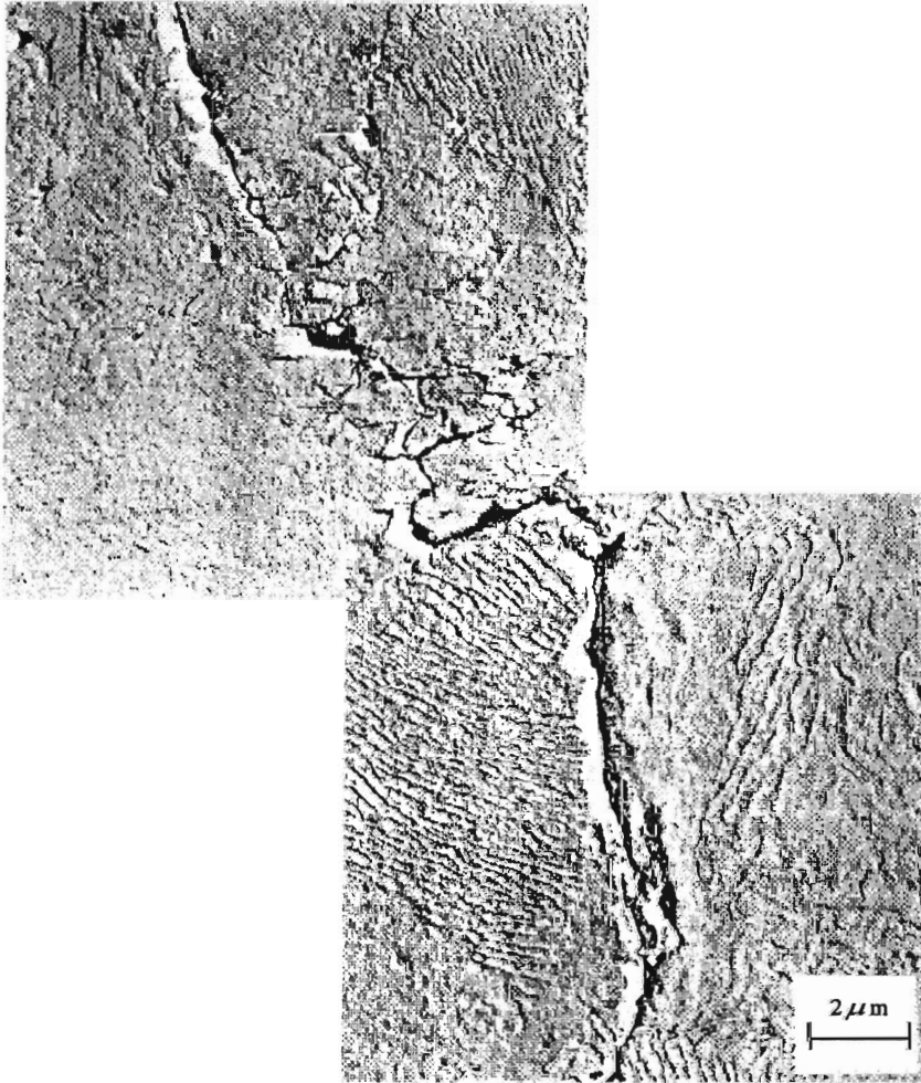
Fig. 4. Path of a surface crack running through a ferrite grain (upper image) and along a pearlite grain boundary (lower image)
