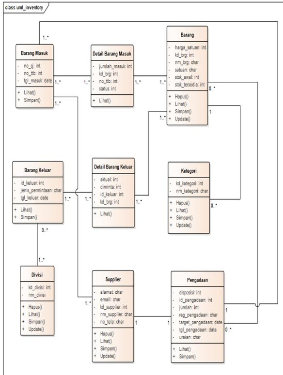
Figure 5. Class Diagram
