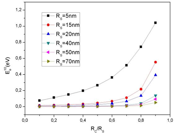
**Figure 2: The energy ground state of an electron inside a core/shell spherical quantum dot drawn versus the core to shell radii ratio  $R_c/R_s$  for:  $F=0 \text{ kV/cm}$  and  $R_s = 5 \text{ nm}$  (Square symbol),  $15 \text{ nm}$  (Circle symbol),  $20 \text{ nm}$  (Up triangle symbol),  $40 \text{ nm}$  (Down triangle symbol),  $50 \text{ nm}$  (Left triangle symbol),  $70 \text{ nm}$  (Right triangle symbol).**
