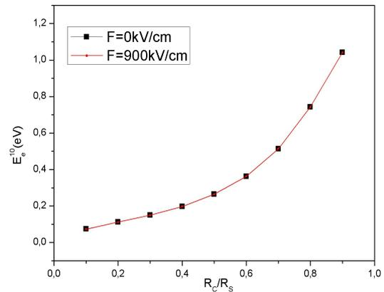
**Figure 3: The energy ground state of an electron inside core/shell spherical quantum dot drawn versus core to shell radii ratio  $R_c/R_s$  for fixed external radius value  $R_s = 5 \text{ nm}$  and various values of the electric field strength:  $F=0 \text{ kV/cm}$  (Square symbol),  $F=900 \text{ kV/cm}$  (Circle symbol).**
