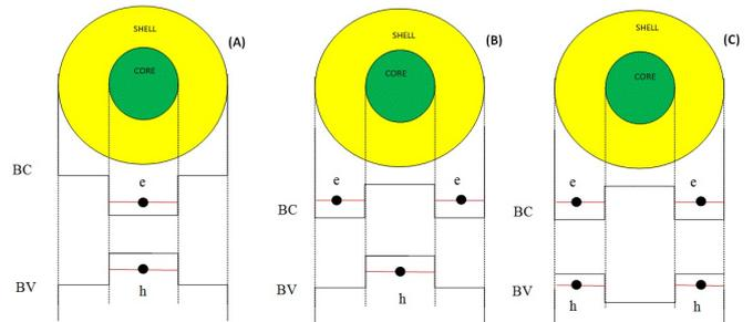
Figure 1: Categories of semiconductor core/shell QD (A) type-I, (B) type-II, (C) reverse type-I.
