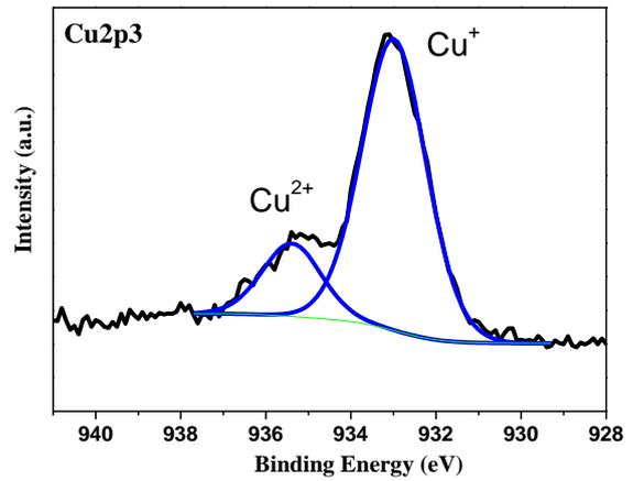
Figure 5: High resolution Cu2p x-ray photoemission spectrum of HCF-NT.
