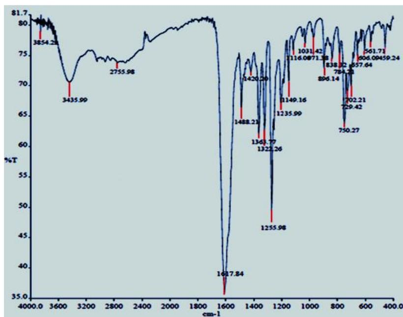
Figure 1. FTIR spectrum of the ligand.
