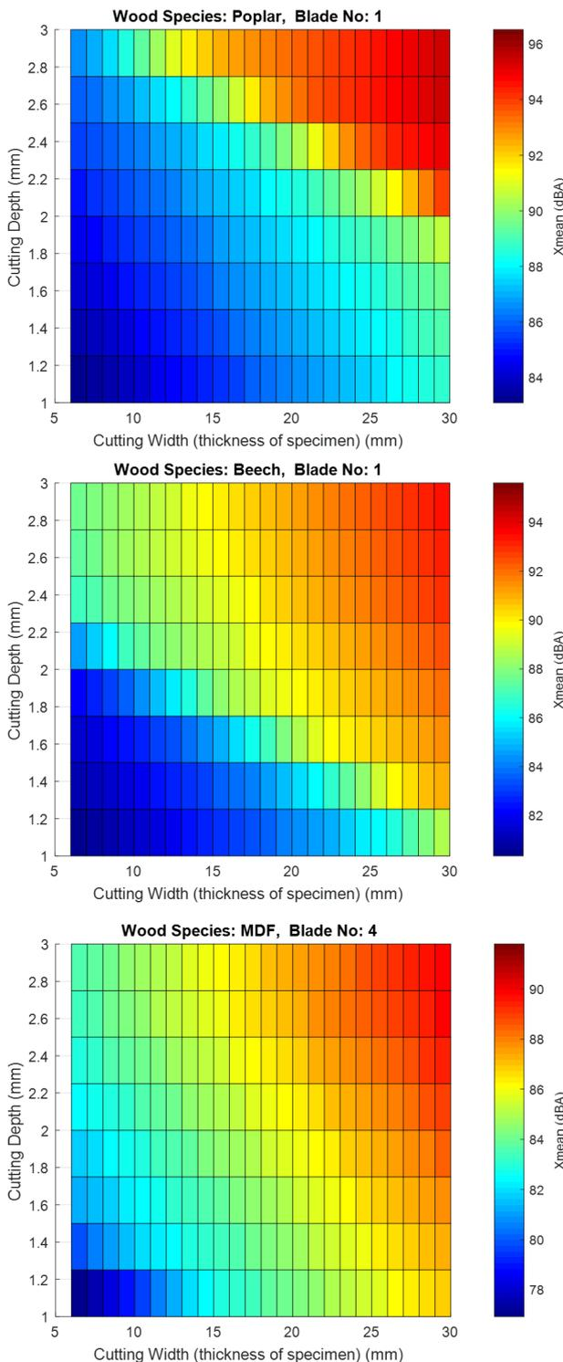
FIGURE 4: Predictive changes in noise emission for different cutting widths and cutting depths.
