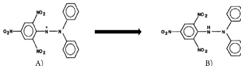
Figure 1. Reaction of an antioxidant with DPPH (Molyneux, 2004); (A) Diphenylpicrylhydrazyl + Antioxidant-OH (Purple color); (B) Diphenylpicrylhydrazyl + Antioxidant-O (Yellow color)
