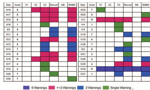
Figure 1: Detailed information of alarm signals generated by control bar matrix (No-alarm days were omitted).
