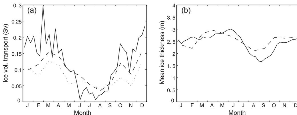
Fig. 1. Mean annual cycle of the Fram Strait (a) ice volume transport and (b) mean ice thickness estimated from the model run (1993–98) (solid line) and from Vinje et al.'s (1998) observations (1993 to July 1996) (dashed line). Also shown in (a) are Kwok & Rothrock's (1999) transport estimates (dotted line).
