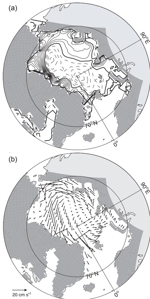
Fig. 4. Arctic (a) ice thickness anomaly (m) at the end of September 1994 and (b) ice velocity in August 1994. In (a) the anomaly is calculated with respect to the mean annual cycle and the contour increment is 0.25 m. Solid isolines indicate positive values; dashed isolines indicate negative values. The bold line is the isoline zero. Also shown in (a) is the model section which has been used for transport estimates in Fram Strait. The dark grey shaded area is the model domain.
