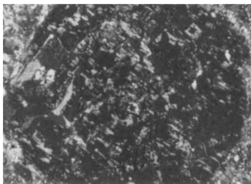
Fig. 6. Rounded phenocryst with intergrowth of plagioclase (white) and potassium feldspar (dark) in clast porphyry from Lilljeborgfjellet. Note jagged border of the phenocryst due to recrystallization of the groundmass. 13 \times .
