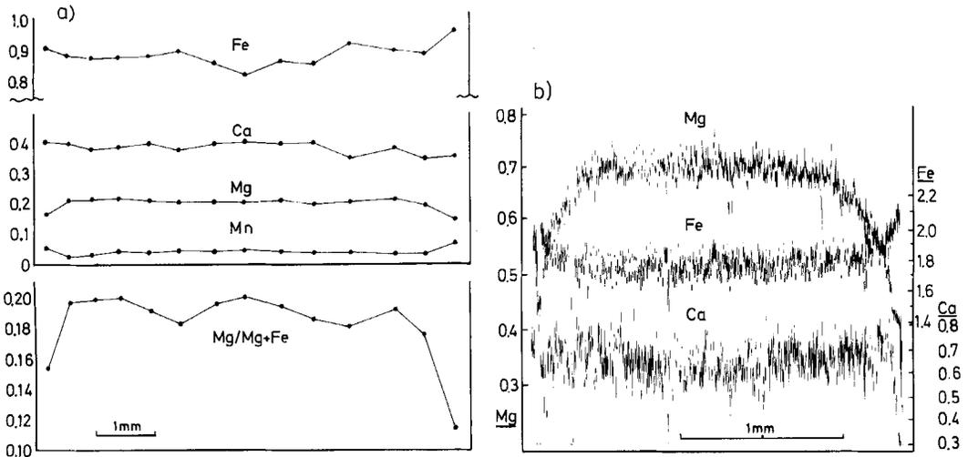
Fig. 3. Compositional profiles of garnets: a) from a garnet amphibolite (BT24, ref. Tables 3 and 4), eastern part of Jutulsessen; b) from a garnet biotite gneiss (ref. Tables 2 and 3), northern Medmulen, eastern Gjelsvikfjella.
