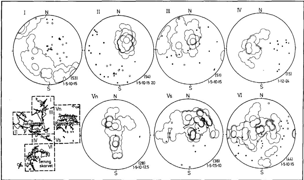
Fig. 5. Stereographic projections, lower hemisphere, of foliations and lineations from Gjelsvikfjella. Division of the subareas and general structures are shown in the inserted map. ( ): number of measured foliation poles; 1-5-10: percentage of the contours for the foliation plots; solid dot: mineral lineation; open circle: fold axis.
