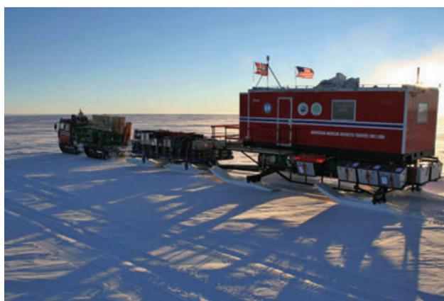
The four tracked vehicles each pulled two sleds loaded with fuel, equipment, and living and working quarters. (Top photo by Atsuhiko Muto. Bottom photo by Stein Tronstad; courtesy of Norwegian Polar Institute Photo Library.)
