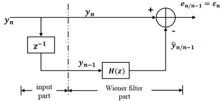
Figure 1: Error Predictor through Wiener Filter
