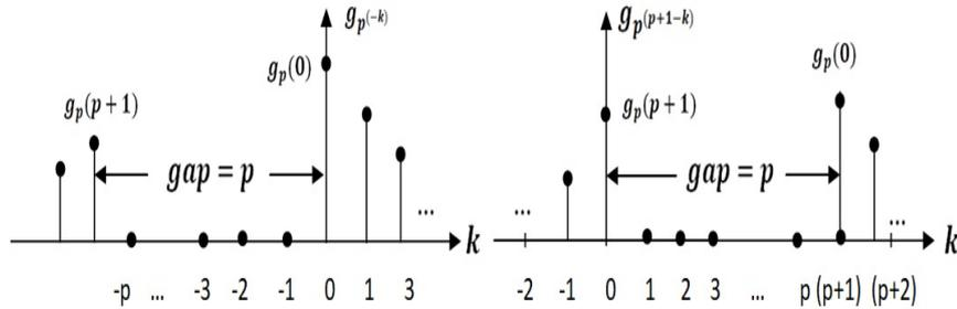
Figure 3: Gap (delay) conditions for  $g_p(k)$  and  $g_p(p + 1 - k)$
