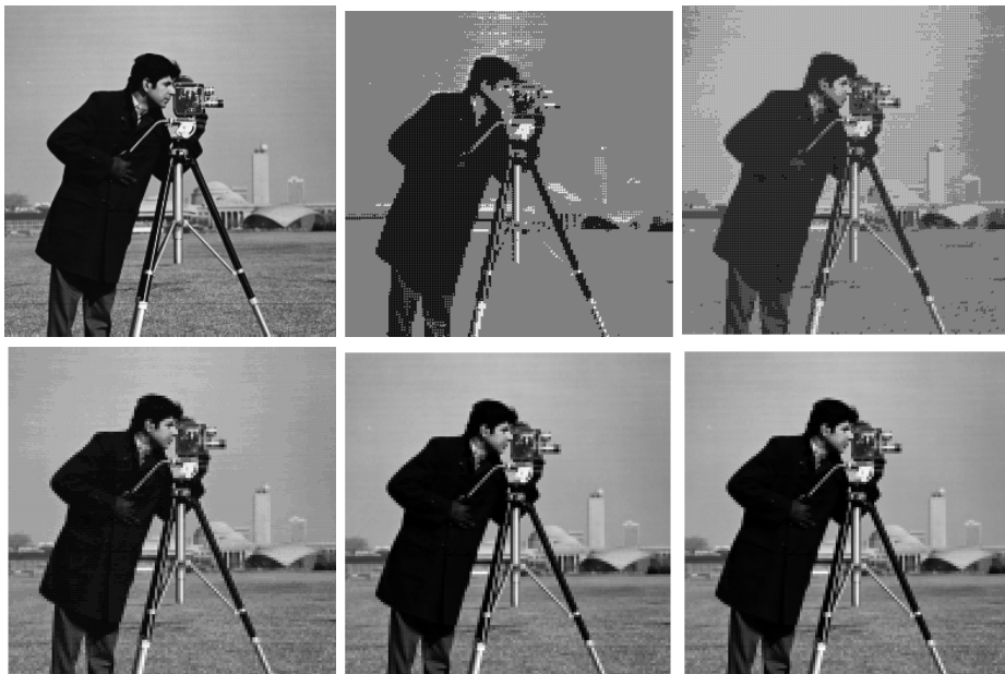
Figure 5: Top left corner: orinal image; left to right: reconstructed Cameraman image using 2 \times 2 blocks at quality indices 5, 10, 50, 90, 95.
