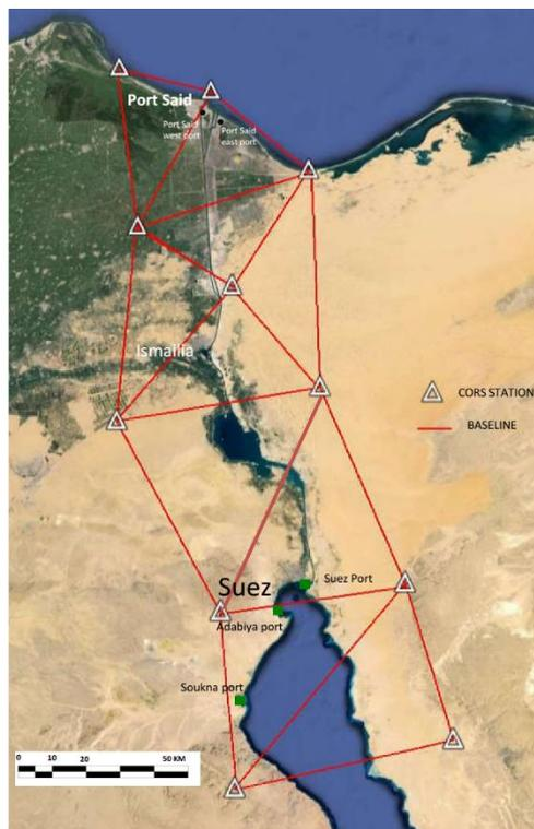
Fig .11 The proposed GNSS network in Suez Canal Corridor Area
