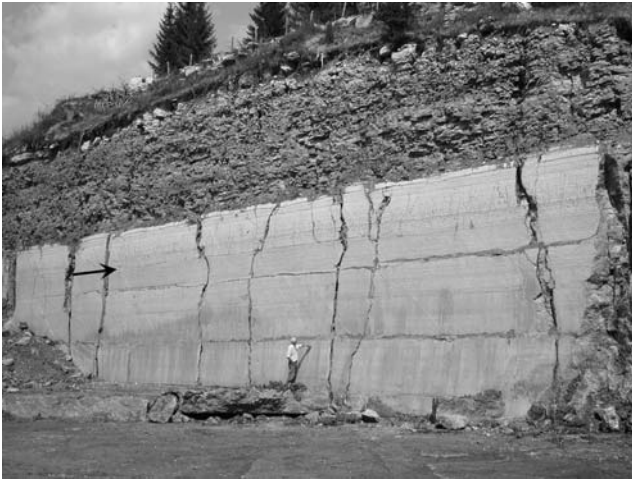
Fig. 3 - Kaberlaba quarry. Temporarily abandoned front where the lower and middle units of the Rosso Ammonitico Veronese are clearly distinguishable. The quarry floor corresponds to the top of the Calcari Grigi. The arrow points to the boundary between the mineralized and the bioclastic facies.
