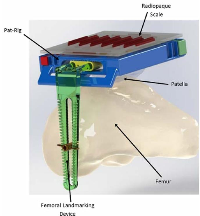
**Figure 4.** Schematic representation of the final design of the Pat-Rig overlaid on the 3D-reconstructed patella and the femur. The radiopaque scale and the Pat-Rig were overlaid on the entire set-up. In silico tests were performed on this set-up and the graft insertion landmarks were accurately marked.
