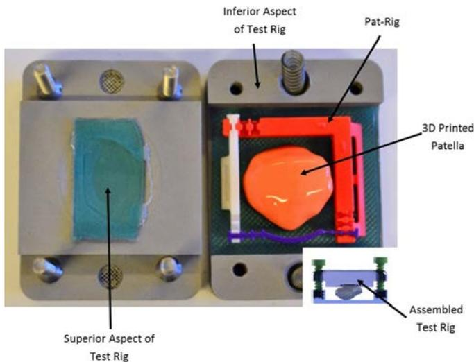
**Figure 5.** Schematic representation of the 3D-manufactured test rig for the Pat-Rig. The device and the 3D-printed patella were stuck together in place using silicone double-sided adhesive. A mechanical drill was used to drill into the patella through the device.
