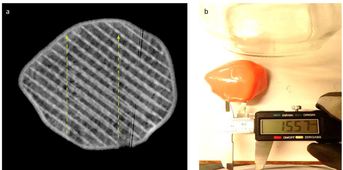
**Figure 6.** (a) X-ray images showing the parallel holes drilled into the 3D-printed patella during bench testing using the test rig. (b) The parallel holes were observed to lie at surgically acceptable distances from each other.
