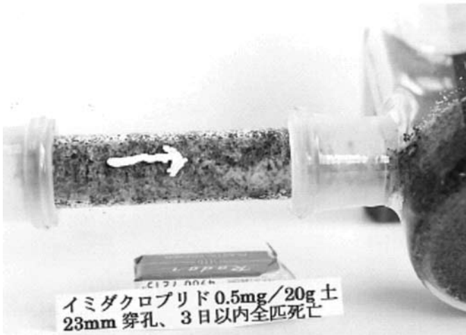
Fig. 4. Typical appearance of the soil in the tunneling test of a non-repellent termiticide. About 20 dead termites were found in the boring.
