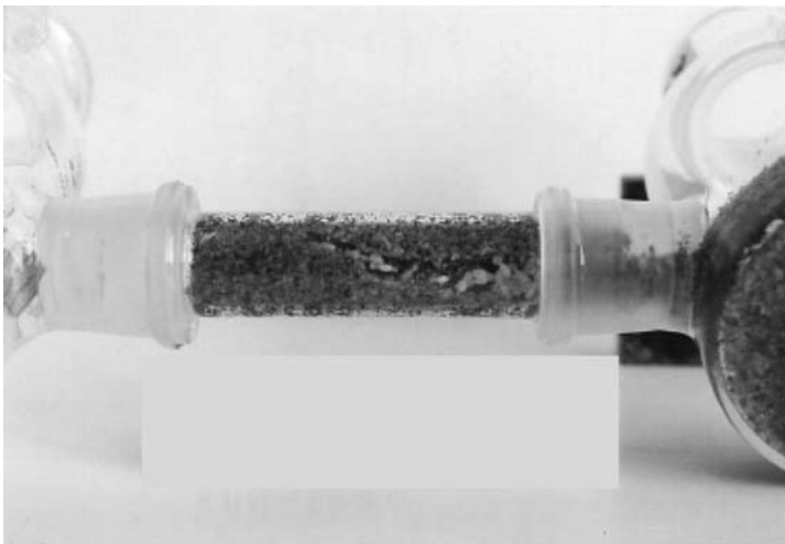
Fig. 5. Typical appearance of the soil in the tunneling test of a non-repellent termiticide. About 18 dead termites were found in the boring.
