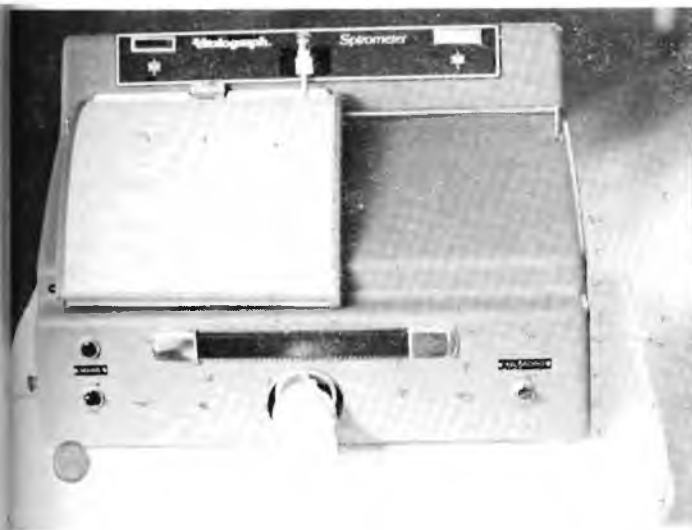
Fig. 3. A Vitalograph single-breath, wedge-bellows, dry Spirometer.
