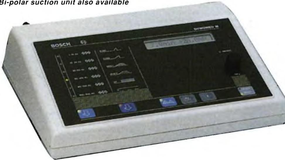
For pain therapy and vegetative changeover, DYNOMED M offers medium-frequency currents, ultra-stimulatory current, and direct current. Also available for rehabilitation are two pulse currents and two modulated swelling currents. Bipolar current application is advantageously performed. The medium frequency currents can also be applied in single-phase mode, ie. with a galvanic component for metabolic stimulation.
