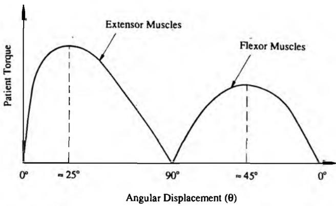
Fig 2: Typical torque versus angle characteristics for the knee joint
