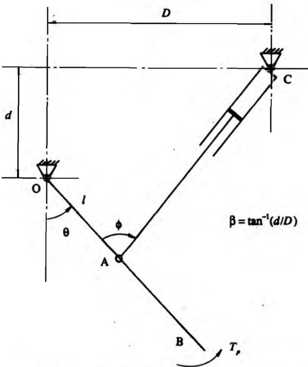
Fig 3: Schematic representation of the proposed exerciser
