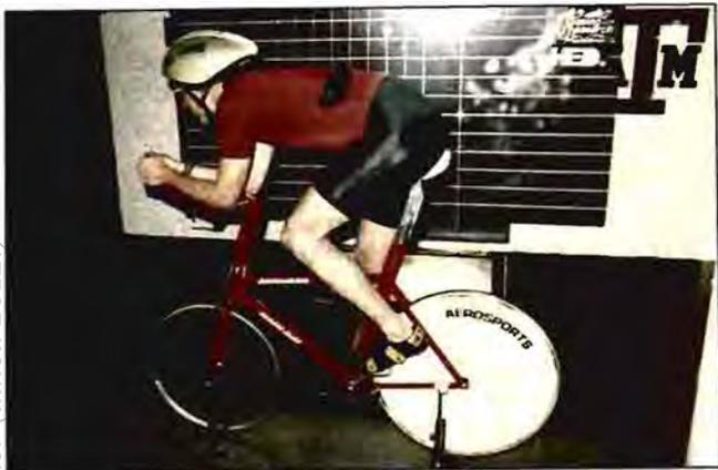
**Figure 5.** Wind tunnel testing of bicycles lead to the development of the time trial funny bike in 1984. The photo shows the Texas A&M wind tunnel, and the bicycle that was used to set the World Amateur Hour record (John Frey USA, 49.946 km; Oct, 10, 1991).
