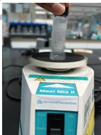
Fig. 5- Preparation of demulsifier DB using Barnstead Thermolyne Maxi Mix II Vortex Mixer
