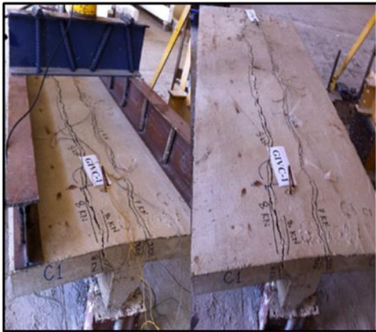
Figure 21. Mode of failure of specimen GIVC-1.
