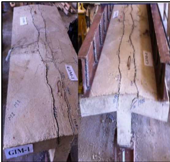
Figure 15. Mode of failure of specimen GIM-3.
