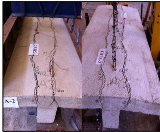
Figure 17. Mode of failure of specimen GIIA-1.
