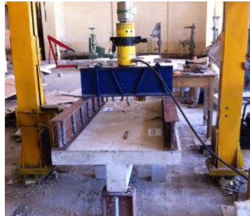
Figure 2. Set-up of the T-beam section in the experimental program.
