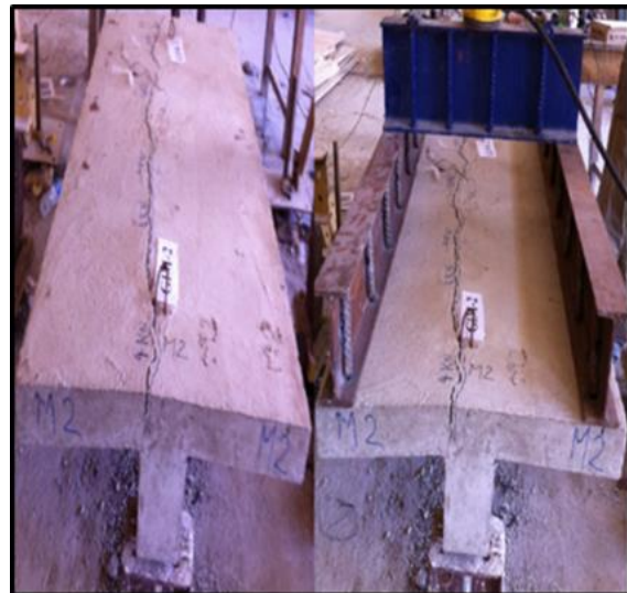
Figure 14. Mode of failure of specimen GIM-2.
