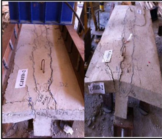
Figure 20. Mode of failure of specimen GIID-2.
