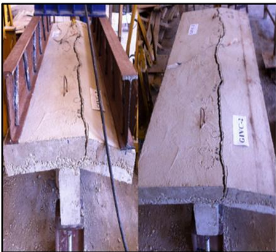
Figure 22. Mode of failure of specimen GIVC-2.
