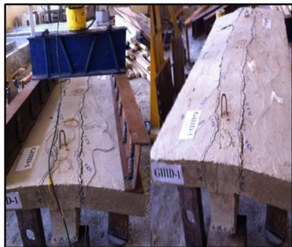
Figure 19. Mode of failure of specimen GIID-1.
