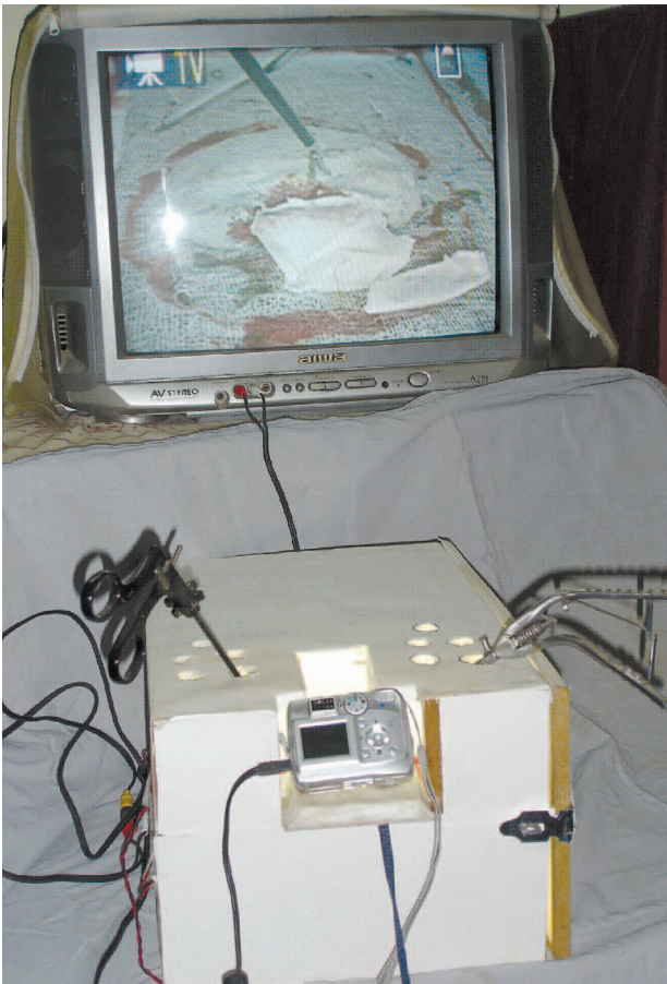
Figure 3. Laparoscopy trainer coupled with a TV monitor.
