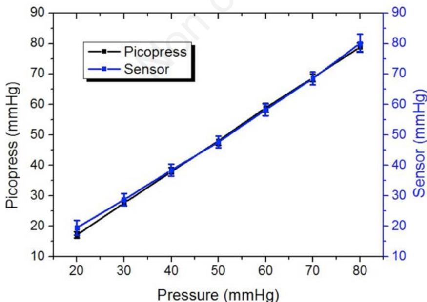
Figure 1. Iontronic sensor versus PicoPress® performance characterization.
