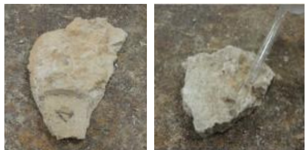
Figure 5. Test with application of hydrochloric acid in some of the samples
